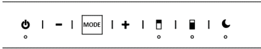
Fig. 5 - Mode Button will display Electronic Controls Fault Codes
