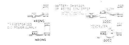
4. NEVER USE A COMMERCIAL 12 VOLT DC TO 120 VOLT AC, 60 HERTZ INVERTER OR CONVERTER, ALSO ENGINE GENERATOR OF NO FREQUENCY CONTROL TYPE for operating your refrigerator on AC, since these devices do not hold the required constant frequency. In case of engine generator frequency control, it must control output with in  $60 \pm 0.5$  hertz.
